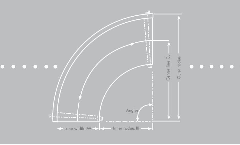
The belts run via idler pulleys, which can lead to a failure in case of a parcel jam on these curves. As a result, not only the belt, but also the expensive idler pulleys will have to be replaced.
